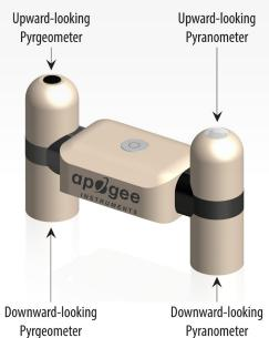
Apogee Instrument's four-component net radiometer consists of an upward-looking and downward-looking pyranometer (to measure shortwave radiation), and an upward-looking and downward-looking pyrgeometer (to measure longwave radiation). Each provide separate measurements of the four components of net radiation.
